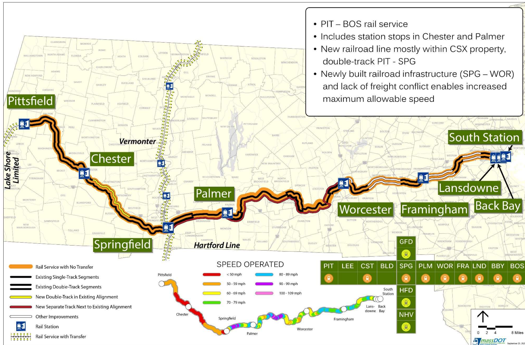
Figure 1-4 – Final Alternative 4 – Passenger Rail, Pittsfield – Boston: Upgraded Existing Rail (PIT – SPG), New Rail in CSX Corridor (SPG – WOR)
