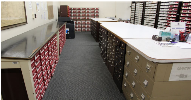
The records are mostly located within reach ranges, except for those on the bottom, but the tables are too high to be usable for someone in a wheelchair.
