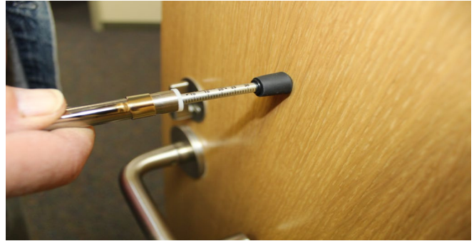
Doors that require more than 5 lbs. of pressure are not compliant.
