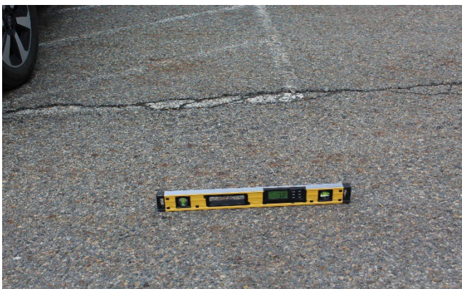
The slope of the parking lot exceeds ADA maximums.
