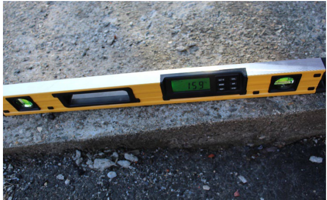
The ramp to provide access into the building is significantly steeper than the ADA limits.
