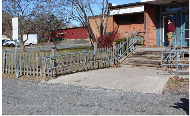
The Spitzer Center is home to the Council on Aging. The accessible parking space sign and lines are faded and there is a change in level from the parking lot to the accessible walkway.
