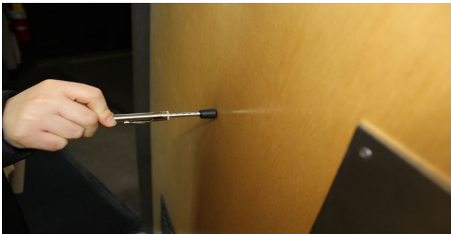
The doors to the bathrooms require approximately 10 lbs. of pressure.
