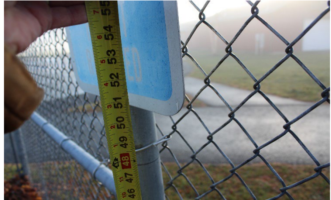
The signs measure at 50.5 inches above the ground, which is below ADA requirements.
