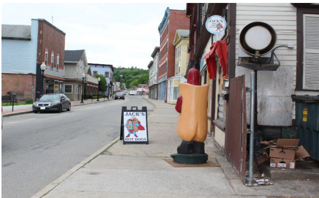
Street furniture should be located on the ground, as shown above, or less than 27" off the ground to be detectable by a cane.
