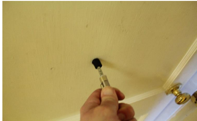
A door pressure gauge measured the amount of effort to open the accessible bathroom door at approximately 15 lbs., which is above the 5 lbs. standard.
