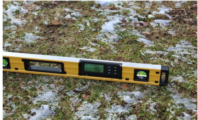
The slope from the parking lot to the playground exceeds ADA standards.
