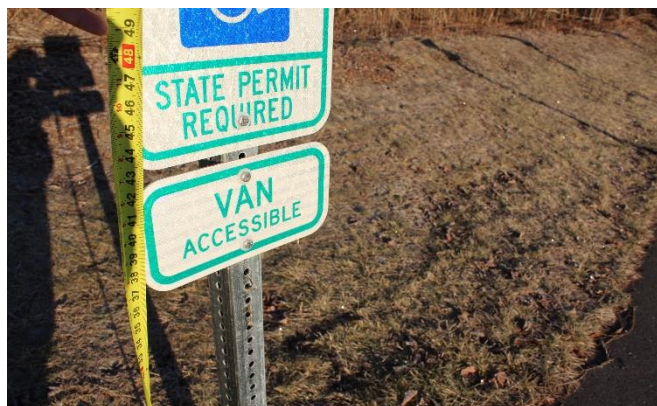
The signs for accessible parking near the baseball and softball fields are too low.
